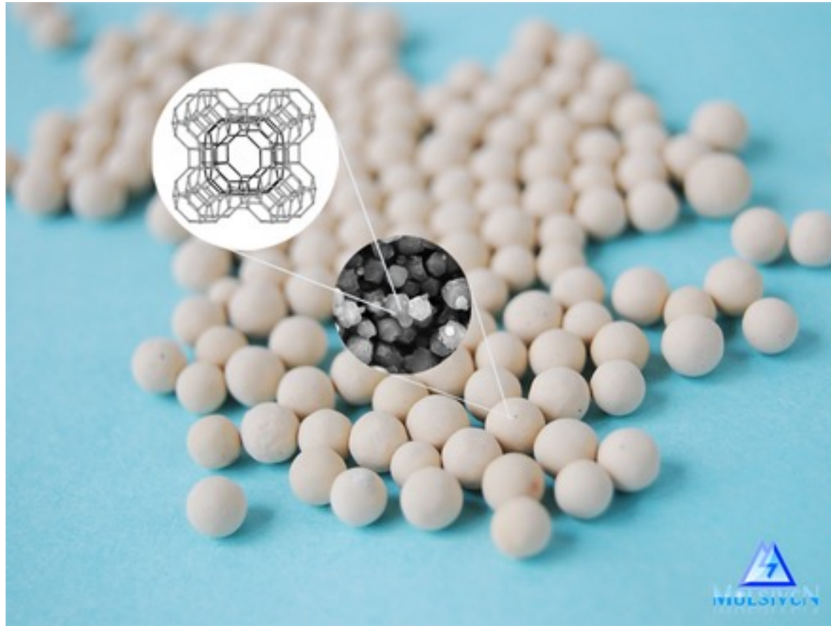
Zeolite as a molecular sieve [16]
